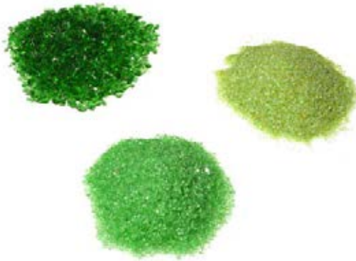
Grain de AFM (activated filter média)
